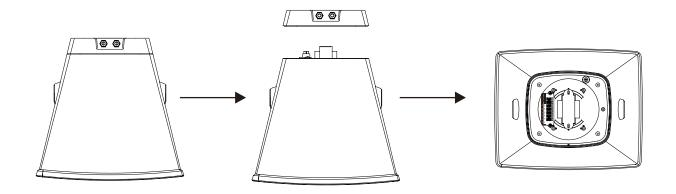
3. Match the horn with the bracket (Step 1 screw), adjust the angle as needed, and then tighten the bracket
