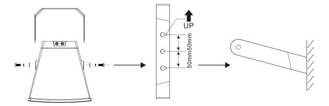
2. Remove the horn back cover, wire as required, and replace the back cover.
